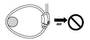
III Do not package in a bent state
